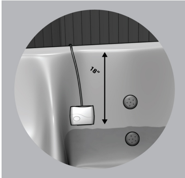
Gently pull cord from cell up over edge of spa at fold in spa cover.
